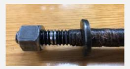
Figure 3: Image of offending bolt/nut assembly showing thread damage
